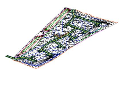
For earthworks we can set-out directly from the design Digital Terrain Model (DTM). This method of setting-out allows the direct measurements of cut or fill from any point on the ground surface to the design DTM.
