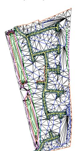
If the setting-out information is readily available in the required format then the whole design can be uploaded into the surveying instrument. This eliminates data input errors, speeds up the setting-out process and reduces the need for manual on-site calculations.
